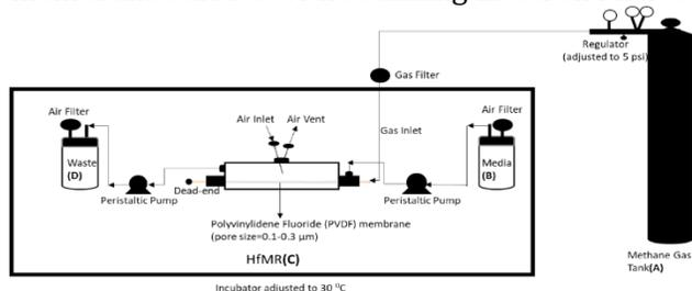
Figure 1: Hollow fiber membrane reactor (HfMR) schematic
