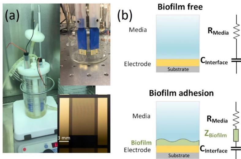
**Figure 1.** Impedance microbiology test apparatus (a) at the CBE to detect *in situ* biofilm growth in aqueous environments. Biofilm growth is detected through electrical modeling of sensor response (b).
