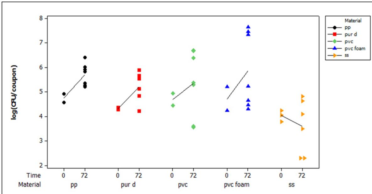
**Figure 1.** Change in bacterial numbers from time 0 to time equal to 72 hours by coupon material type.
