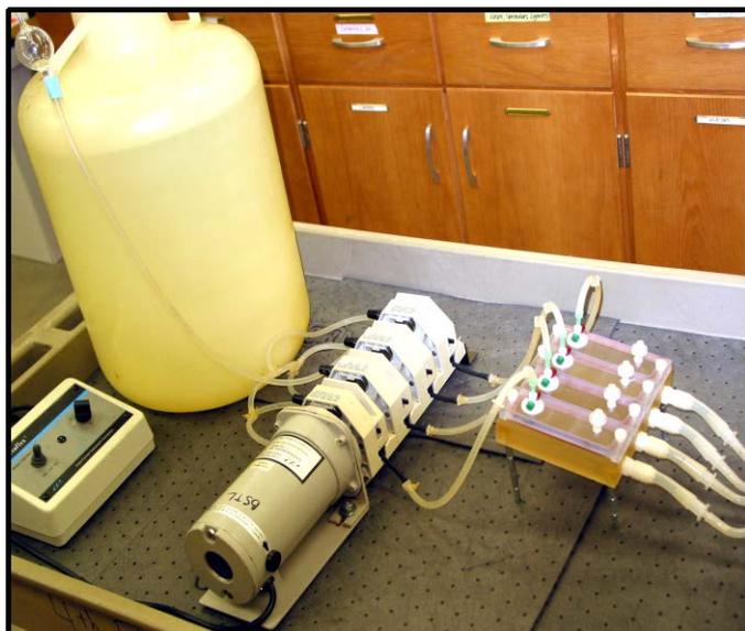
Figure 1. Assembled DRF reactor.
