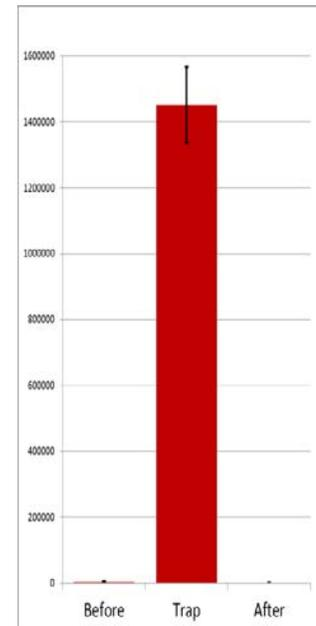
**Fig.1:** Histogram showing the concentrations of bacterial cells prior to the trap, inside the trap, and after the trap using ATP assay. The sample was 500 mL of seawater containing trace *Marinobacter*. Preliminary work indicated that the BiyoTrap concentrates with equal efficiency all Gram-negative and Gram-positive organisms in a variety of liquids including water, PBS, seawater and fuel.
